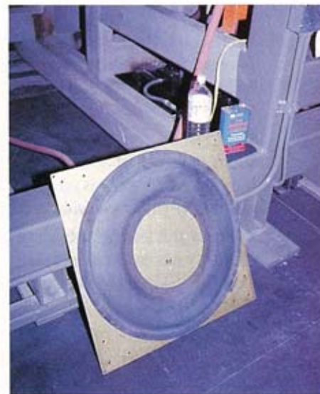
One of the airbags which, when inflated, raises the movable towers so that they 'float' to new positions.
