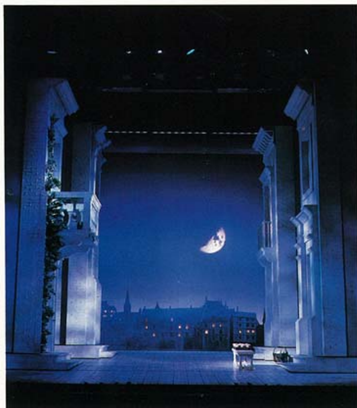
For the Balcony Scene (above left), a three dimensional ground row is used in front of a twin white back projection screen. The black sharktooth gauze is 'clouded' by the upstage Digital Light Curtains. There are cobblestone gobos on the deck and break-ups on the towers, and the actors, when on stage, are lit by a combination of VL5s and R&V beam lights. Cobblestone gobos as used in the Street Scene (above right).
